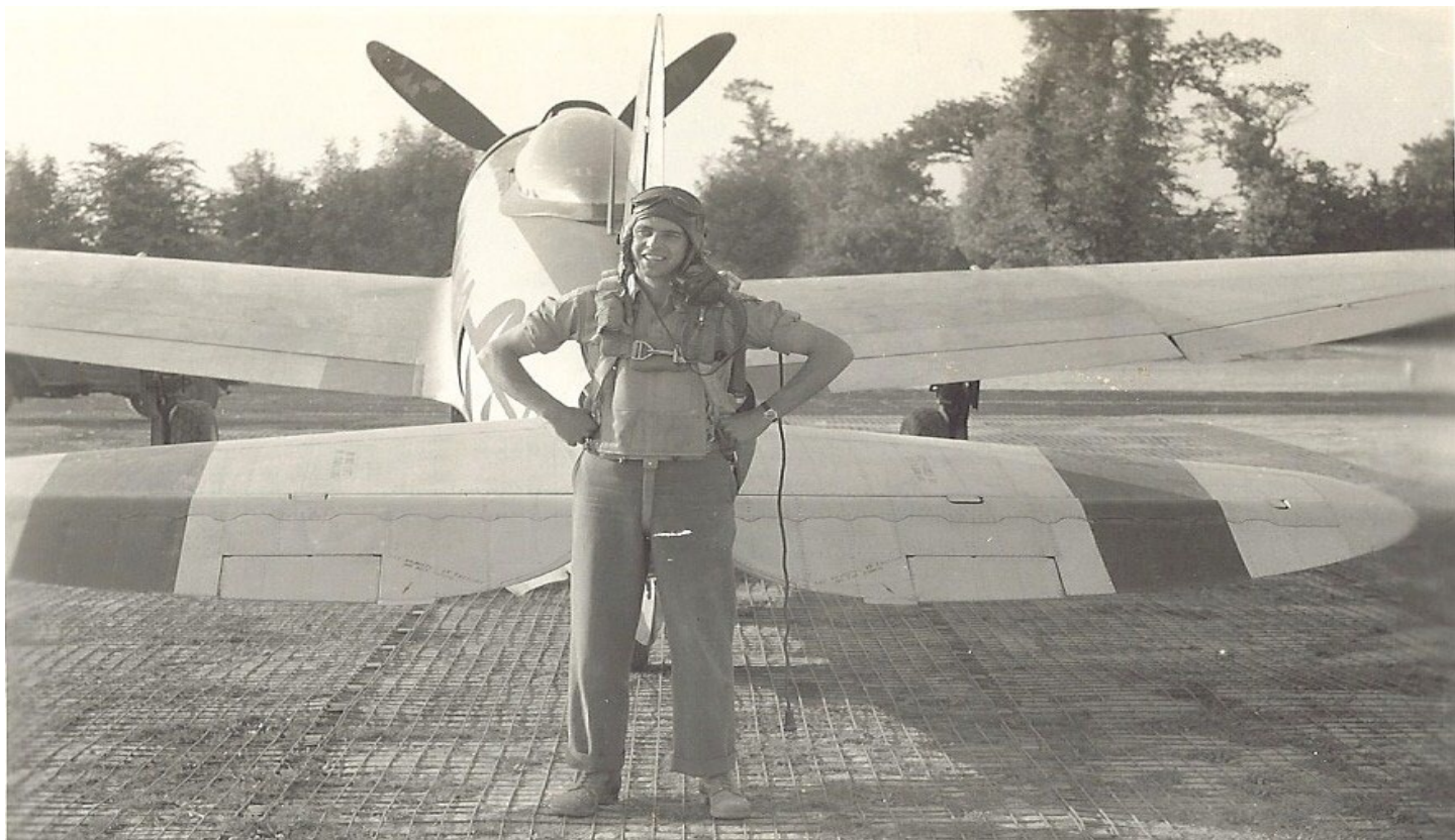
Henry Bakken standing in front of a "bubbletop" Thunderbolt with no camouflage or invasion stripes. Note the metallic lattice layed on the ground, to prevent the nearly 8 tons of the Thunderbolt from bogging down in mud on the hastily set up Advanced Landing Grounds
