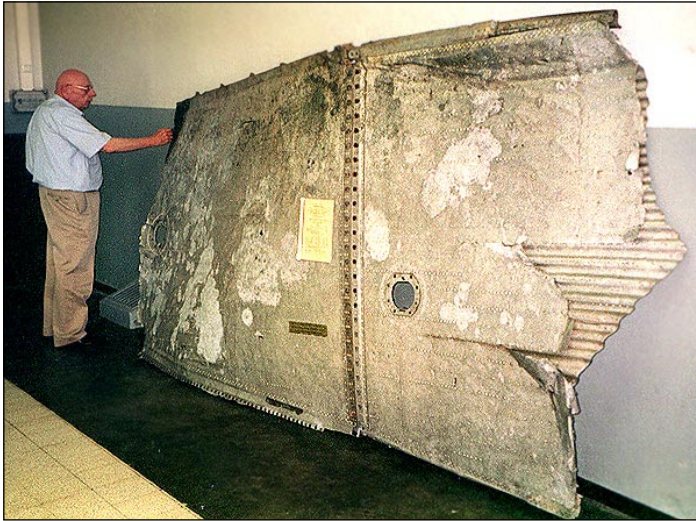
This picture gives an idea of the size of the wing panel. It also shows the joint between the outer and the inner wing (Right hand).
